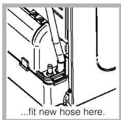
Fit a suitable length of hose to the new location shown (see diagram).
